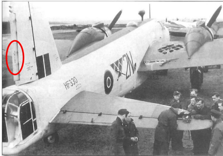
Illustration 13 – Rudder trim tab with 'DO NOT HANDLE' (p55)
